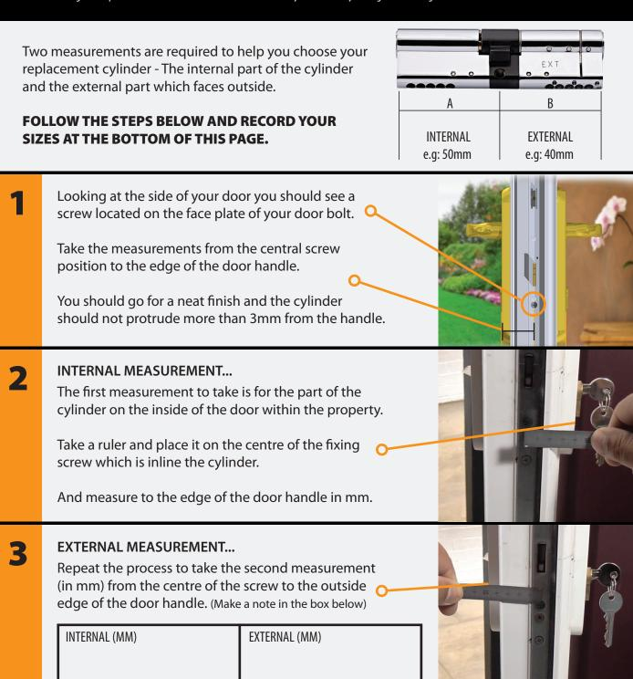
Replacing a Euro cylinder on the vast majority of doors is a simple process. The only tool required is a crosshead screwdriver.
